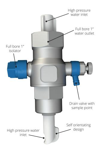
Global Water Solutions' FlowThru™ inline adaptors are ideally suited for continious pressure systems where there is a risk of stagnant water in the tank. The FlowThru™ inline adaptor diverts the water through the tank while the pump is running, eliminating the risk of stagnant water and reducing the risk of waterborne bacteria such as legionella. This constant flushing ensures the freshest water in the tank.
