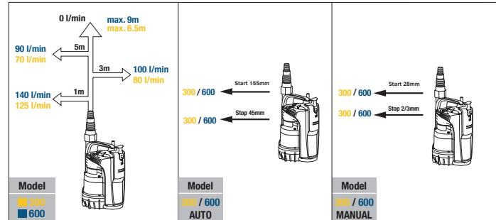
**GB** Submersible pump designed specifically for pits with small size (minimum 20 cm x 20 cm). Suitable for pumping clean water containing particles with maximum diameter up to 5 mm. Very low priming and starting level of the pump 10-15mm (manual mode) and low suction capability down to 2-3 mm.
