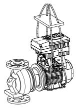
Fig. 2: Transporting a horizontal pump set
