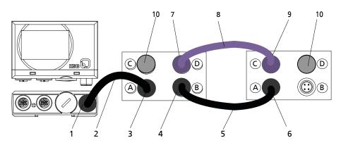
Fig. 39: Connecting PumpMeter in dual and multiple pump configurations
