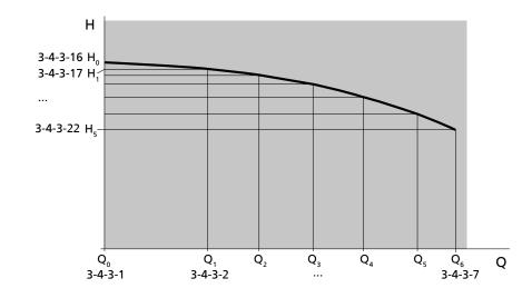
**Fig. 68:** Characteristic head curve with seven data points and the relevant parameters Flow rate  $Q_0$ , i.e. parameter (3-4-3-1), is always zero. Flow rate Q6 (3-4-3-7) describes the end of the characteristic curves and also represents the maximum permissible flow rate of the pump.
