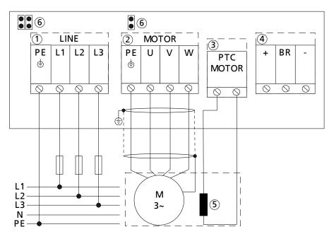
Fig. 16: Establishing the mains power supply and motor connections, size A, 400 V/3~ variant
