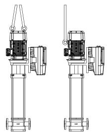
Fig. 3: Transporting a vertical pump set
