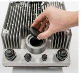
2. Remove the nut from the screw plug inside the frequency inverter.
