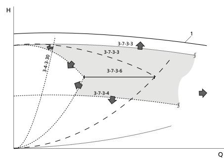
Fig. 67: Switching limits of two running pumps in a multiple pump system
