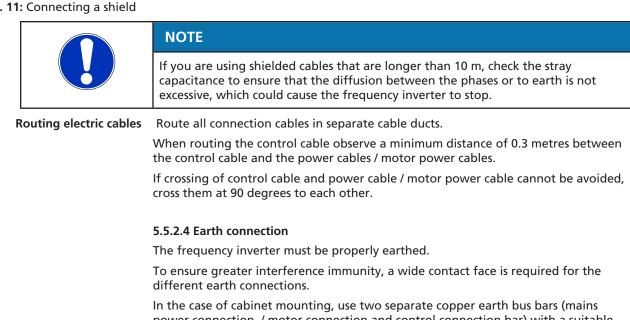
power connection / motor connection and control connection bar) with a suitable size and cross-section for earthing the frequency inverter. All the earth connections are connected to these.
