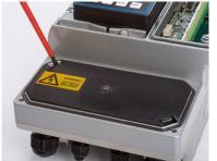
Fig. 13: Prying open the protective cover
