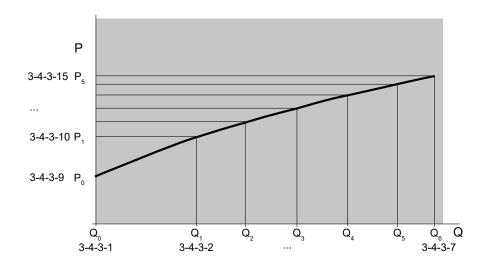
Fig. 69: Power curve with seven data points and the relevant parameters
