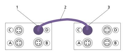
Fig. 37: Connecting M12 modules in dual and multiple pump configurations
