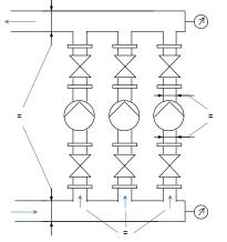
**Fig. 71:** Conditions for improving accuracy with pressure sensors installed close to the pump in multiple pump systems
