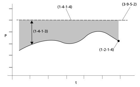
Fig. 80: Energy savings with constant reference power
