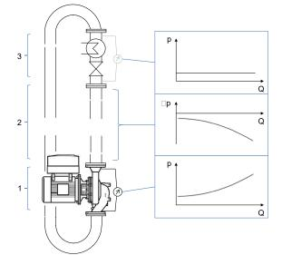
Fig. 73: Differential pressure control with dynamic pressure compensation in closed system
