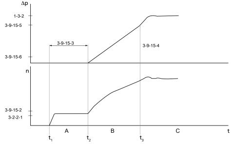
Fig. 86: Pipe filling function time diagram
