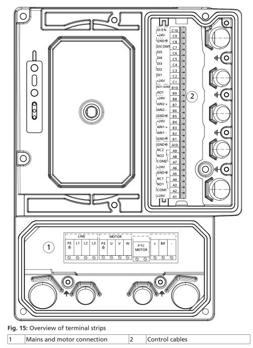
5.5.3.3 Connection to mains power supply and motor
