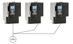
Fig. 32: Establishing an earth connection
