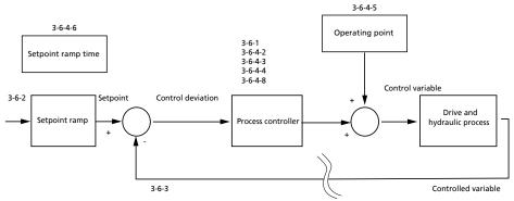
Fig. 63: Overall structure of the process controller
