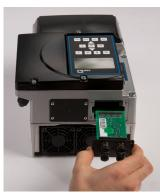
**Fig. 42:** Inserting the field bus module
