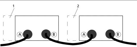
Fig. 44: Connecting the field bus module
