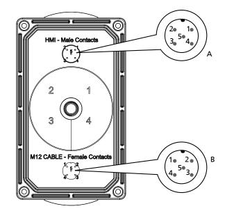
Fig. 54: Pin assignment for M12 connection cable and control panel
