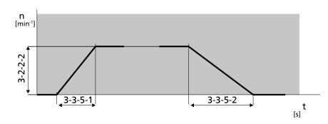
Fig. 82: Start ramp (left) and stop ramp (right)
