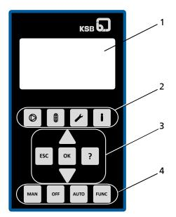
Fig. 55: Graphical control panel
