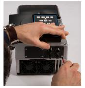
**Fig. 36:** Securing the M12 module
