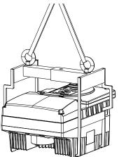
Fig. 5: Transporting the frequency inverter with lifting gear
