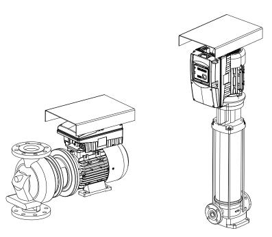
Fig. 9: Pump set with protective roof
