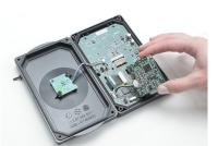
Fig. 49: Installing the Bluetooth module
