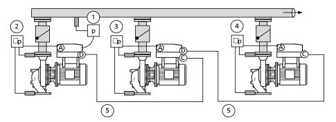
Fig. 92: PumpMeter as internal measured variable source per pump, external pressure sensor as actual value source
