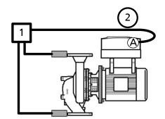
Fig. 91: PumpMeter as actual value source via Modbus
