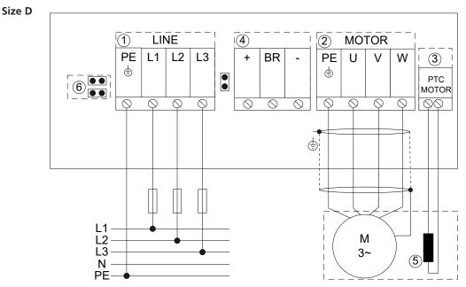
Fig. 19: Connection to mains power supply and motor, size D
