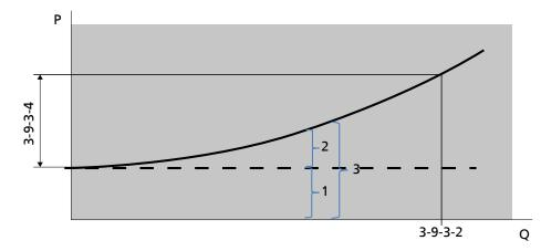
Fig. 78: Setpoint compensation curve for dynamic pressure compensation based on flow rate
