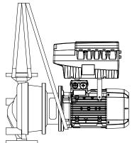
Fig. 1: Transporting a close-coupled pump set
