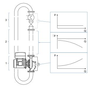
Fig. 77: Differential pressure control with dynamic pressure compensation in closed system
