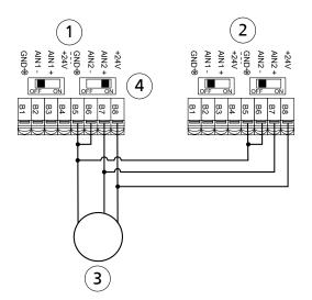
Fig. 88: Example, looping of a 4 - 20 mA signal
