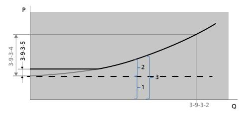
Fig. 75: Setpoint compensation curve for dynamic pressure compensation based on flow rate with minimum setpoint compensation (3-9-3-5)
