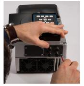
**Fig. 43:** Securing the M12 module
