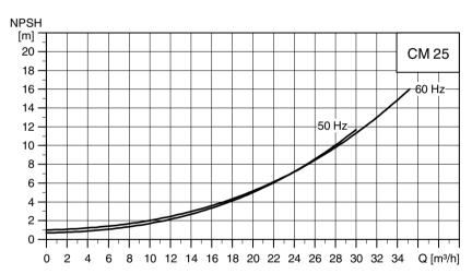
Fig. 9 NPSH curves for CM 25
