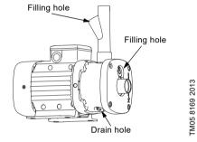
Fig. 11 Position of filling holes and drain hole
