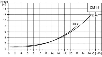
Fig. 8 NPSH curves for CM 15
