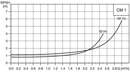
Fig. 4 NPSH curves for CM 1
