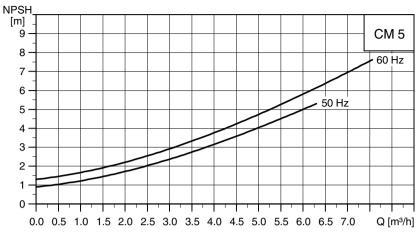
Fig. 6 NPSH curves for CM 5
