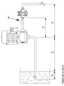
Fig. 4 Recommended pipes for a self-priming pump
