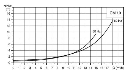
Fig. 7 NPSH curves for CM 10
