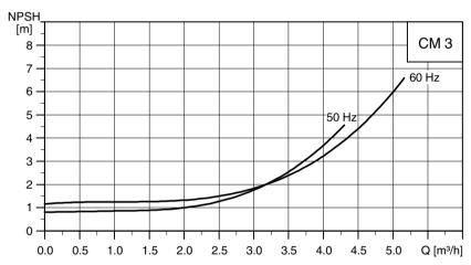
Fig. 5 NPSH curves for CM 3
