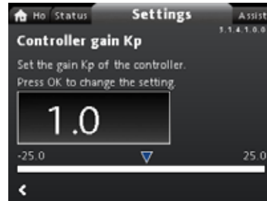
Fig. 60 "Controller gain Kp"
